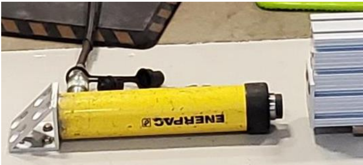
Figure 43: Test setup for the C channel slide test
