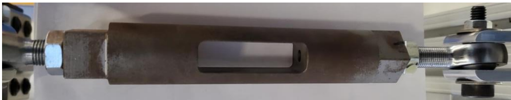
Figure 24: Turnbuckle with an uneven initial rod depth set
