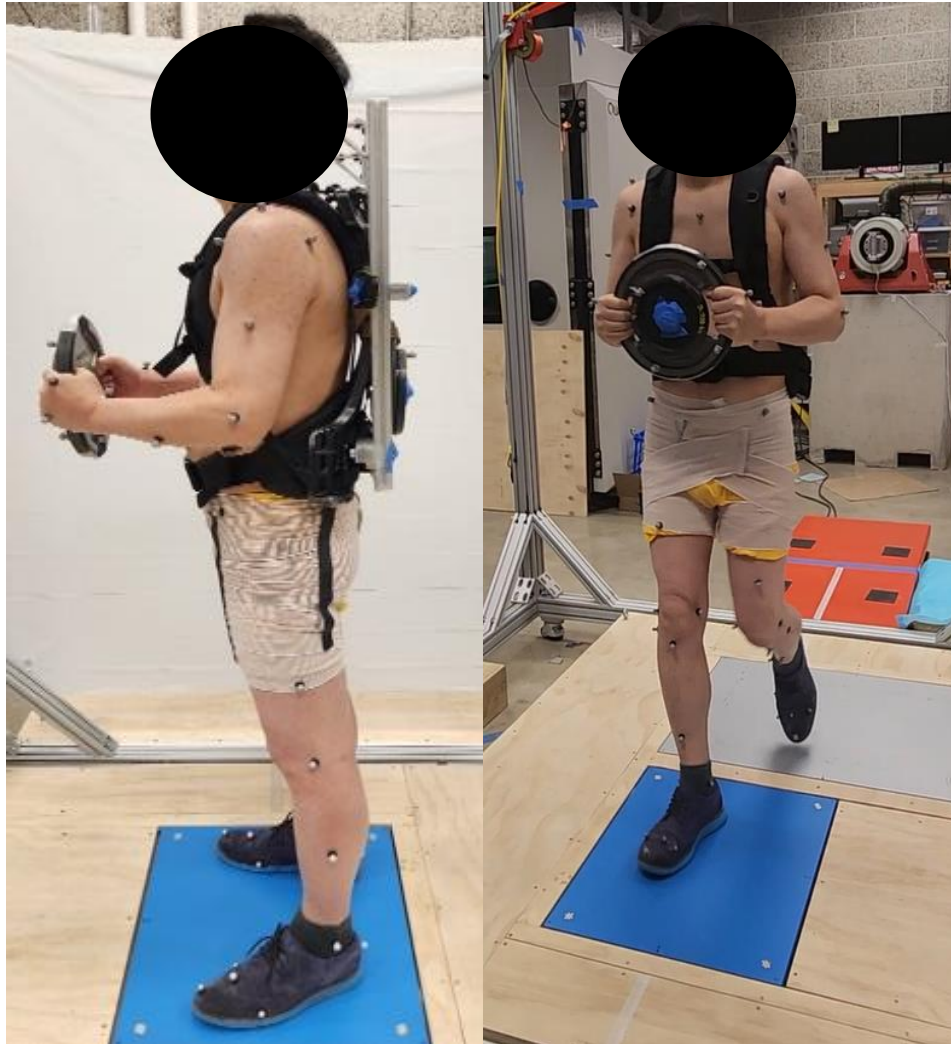
Figure 3.6 Illustration of quiet standing and walking conditions with weight in hands while wearing a mock exoskeleton.
