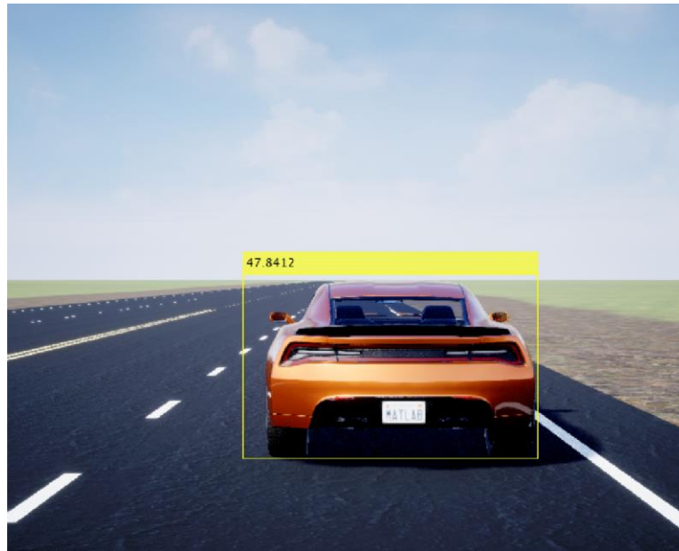
Figure 9: Example of camera image with bounding box, as result of ACF object detector
