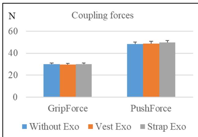
Figure 3.20 Exoskeleton (Exo) effect on mean coupling forces.
