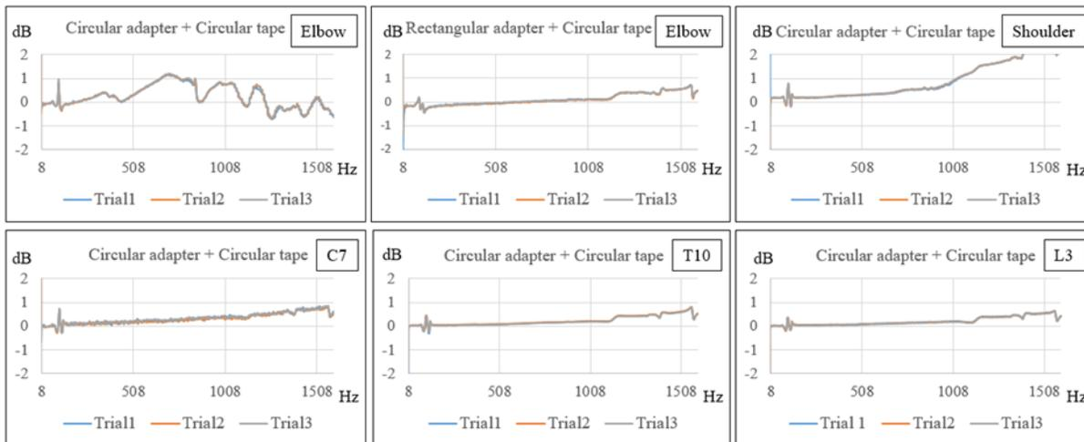
Figure 3.2 Accelerometer adaptor base frequency responses (dB) between 8 Hz and 1600 Hz
