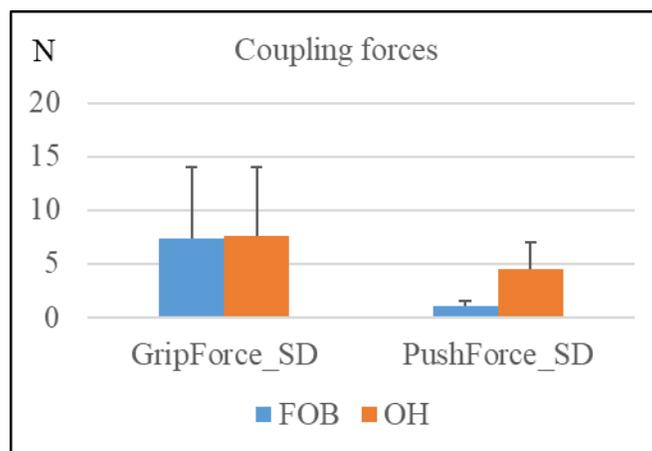
Figure 3.22 Posture effect on peak-to-peak coupling forces. OH: overhead posture; FOB: front-of-body posture.
