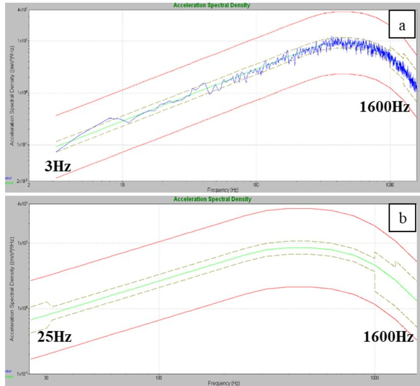
Figure 2.8 Illustration of one testing run of the extended random vibration spectrum (a) and the theoretic spectrum defined in the ISO 10819 (2013) (b).
