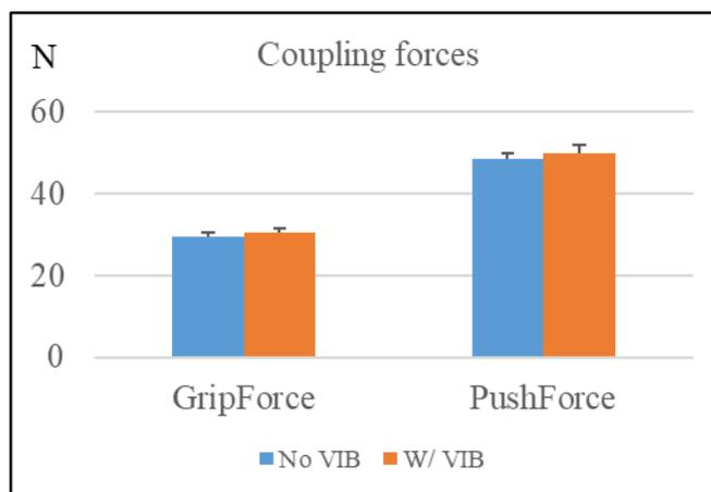
Figure 3.21 Effect of vibration on/off conditions on mean coupling forces
