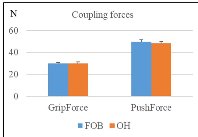
Figure 3.19 Posture effect on mean coupling forces. OH: overhead posture; FOB: front-of-body posture.
