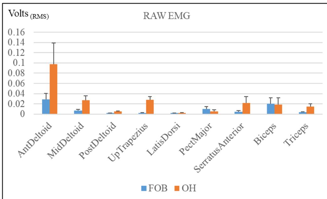
Figure 3.13 Posture effect on raw EMG (Volts in RMS) for 9 muscles. OH: overhead posture; FOB: front-of-body posture.
