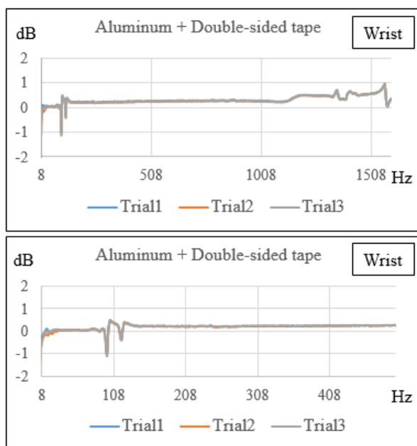
Figure 3.4 Wrist adaptor base frequency response of two frequency ranges from 8 Hz to 1600 Hz (up) and from 8 Hz to 500 Hz (down).
