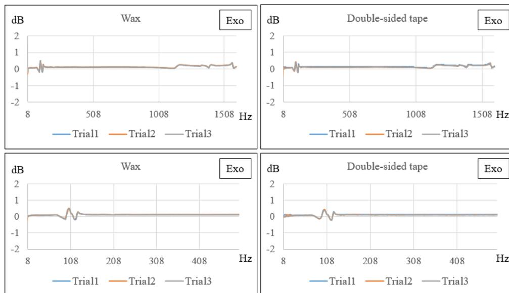
Figure 3.5 Bare accelerometer frequency response at the Exo arm link with two attachment methods for frequency ranges from 8 Hz to 1600 Hz (up) and from 8 Hz to 500 Hz (down).
