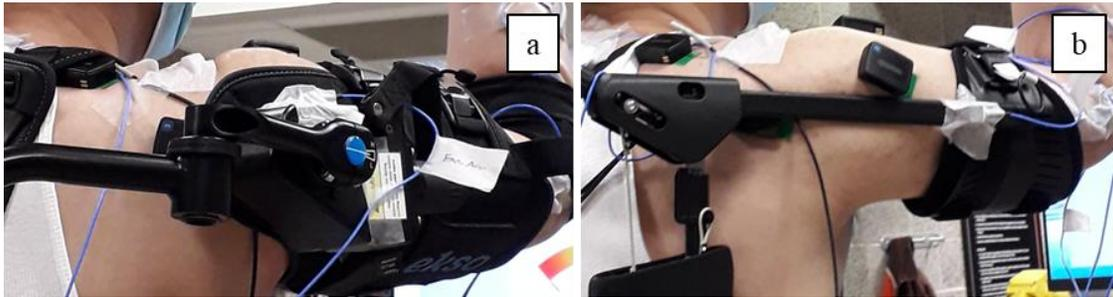
Figure 2.10 accelerometer attachment on exoskeletons' frame Vest-Exo (a), Strap-Exo(b)
