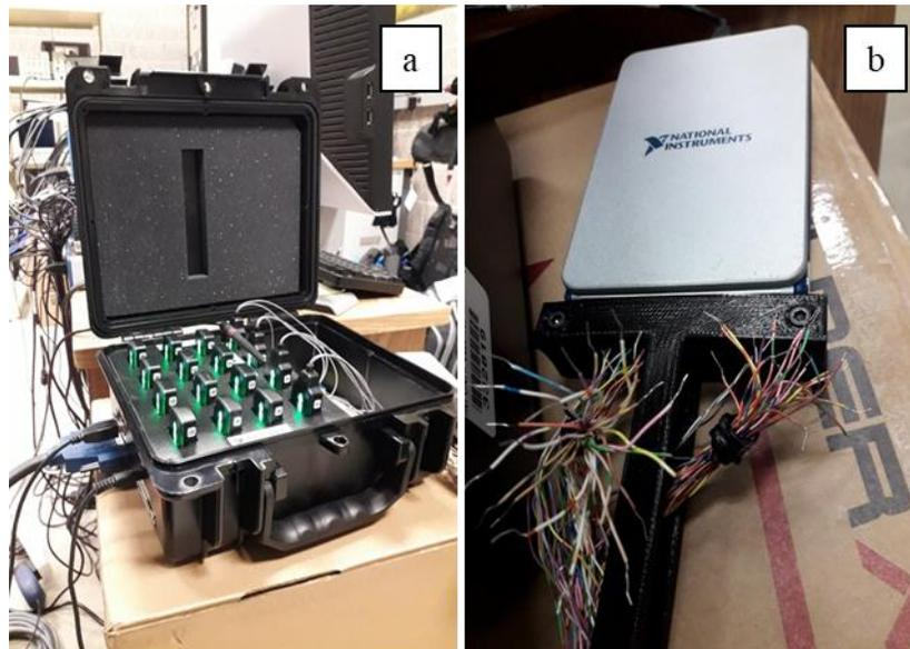
Figure 2.12 The DELSYS Trigno Wireless EMG System (a) and the NI-DAQ 9205 voltage input module (b) for recording muscle activities.
