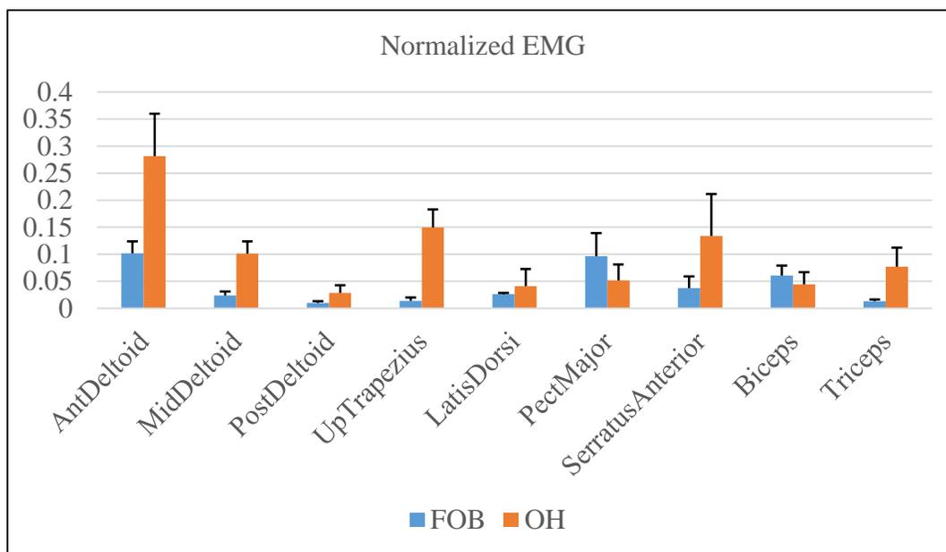
Figure 3.14 Posture effect of on normalized EMG for 9 muscles. OH: overhead posture; FOB: front-of-body posture.
