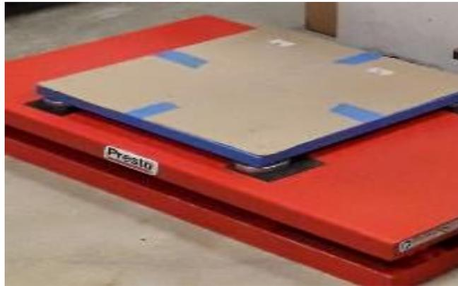
Figure 2.15 A force plate 9260AA and A scissor lift placed under the subject's feet.
