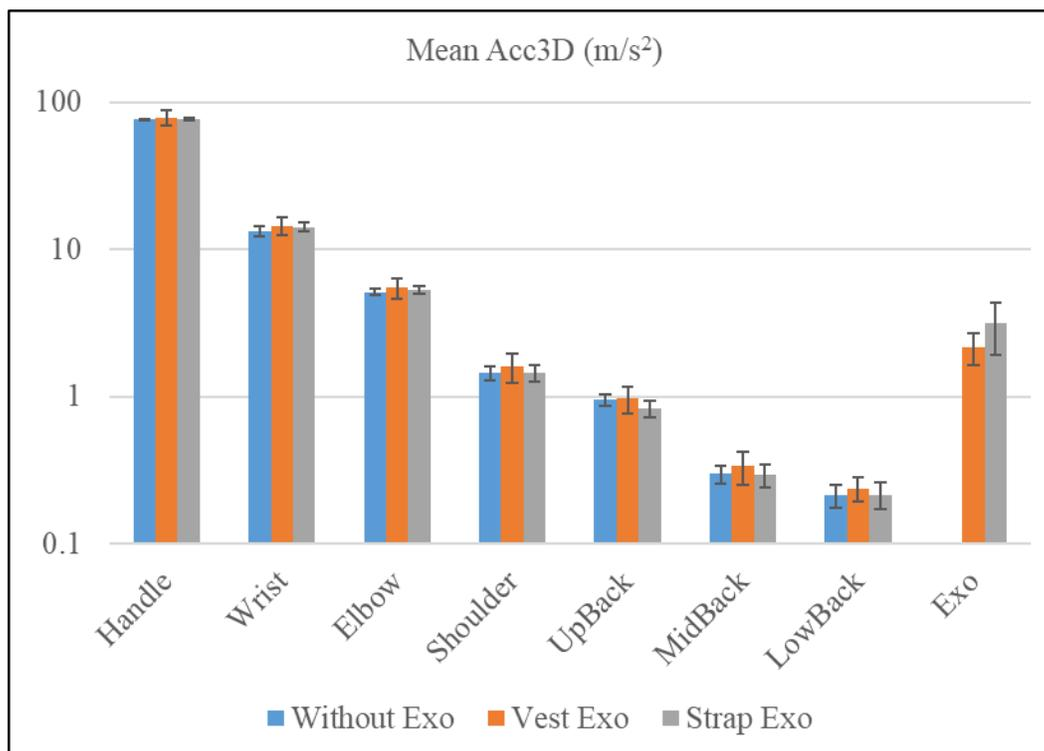
Figure 3.8 Exoskeleton (Exo) effect on mean acceleration magnitude at the shaker handle, six body locations, and the arm link of exoskeletons.
