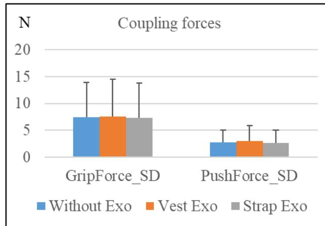
Figure 3.23 Exoskeleton (Exo) effect on peak-to-peak coupling forces.
