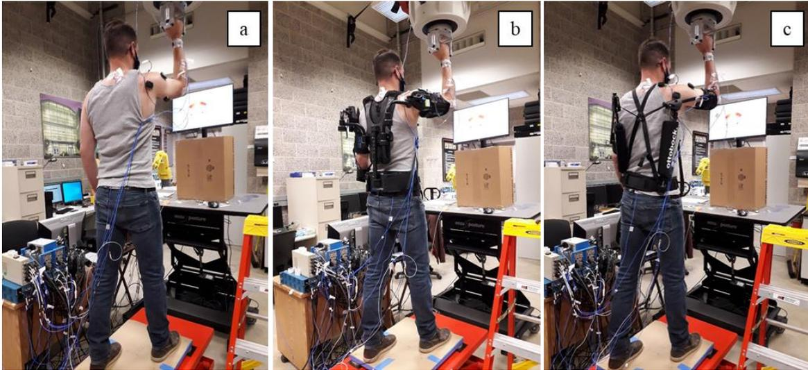
Figure 2.3 Illustration of not wearing exoskeleton (a), wearing a vest-type exoskeleton (b), and wearing a strap-type exoskeleton (c).
