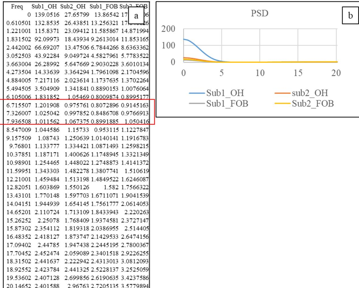
Figure 3.1 Illustration of the shaker PSD handle z-axis amplitude ( $\text{m/s}^2$ ) under 20 Hz, including one example of actual shaker PSD values (a) and exemplary shaker PSD curves for two postures (b).
