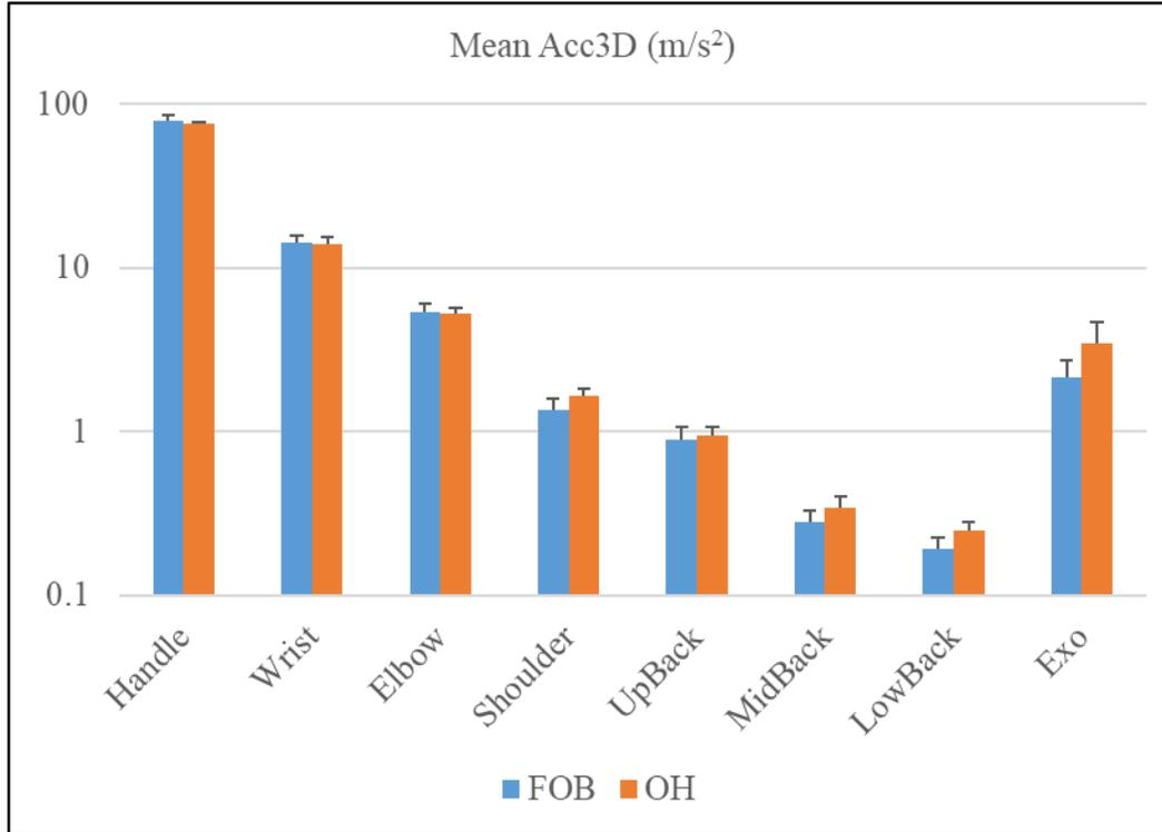
Figure 3.7 Posture effect on mean acceleration magnitude at the shaker handle, six body locations, and the exoskeleton. OH: overhead posture; FOB: front-of-body posture.
