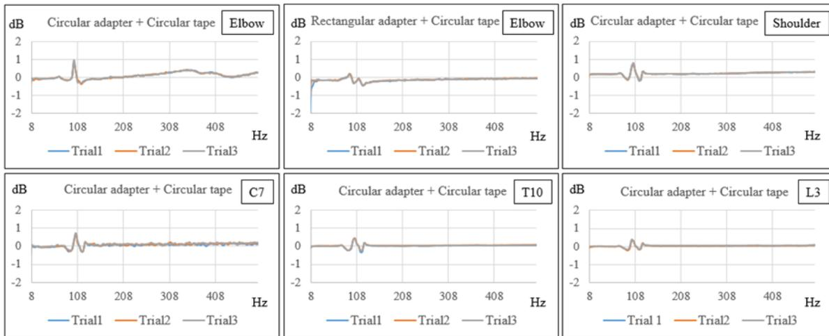
Figure 3.3 Accelerometer adaptor base frequency responses between 8 Hz and 500 Hz.
