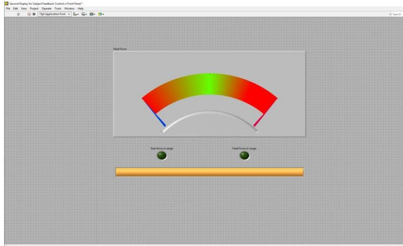
Figure 2.16 Live feedback interface in a LabVIEW environment with the red needle representing grip force and the blue needle representing push force.
