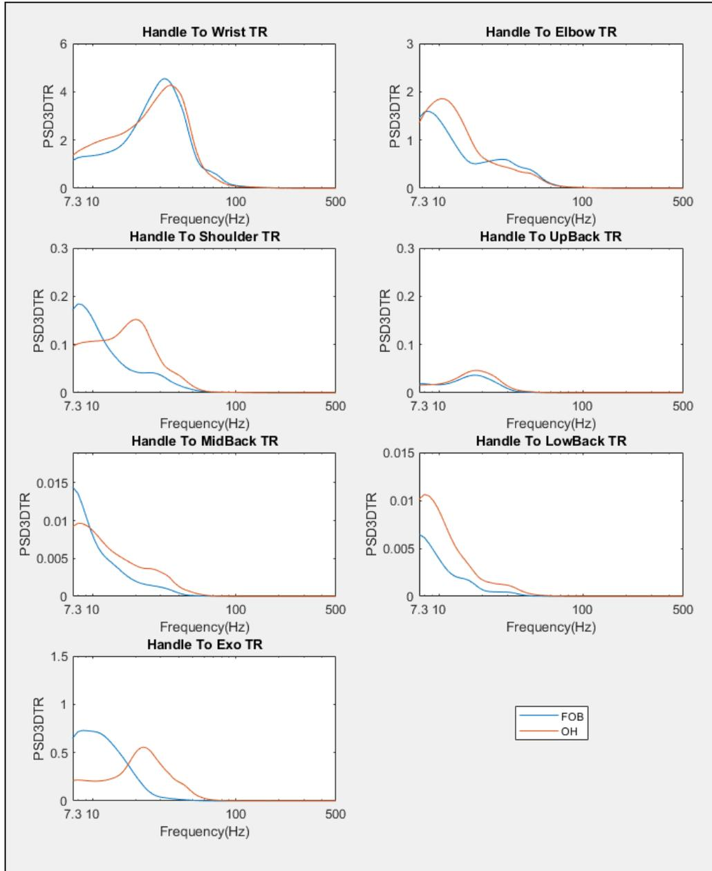
Figure 3.11 Posture effect on PSD transmissibility in the frequency domain. OH: overhead posture; FOB: front-of-body posture.
