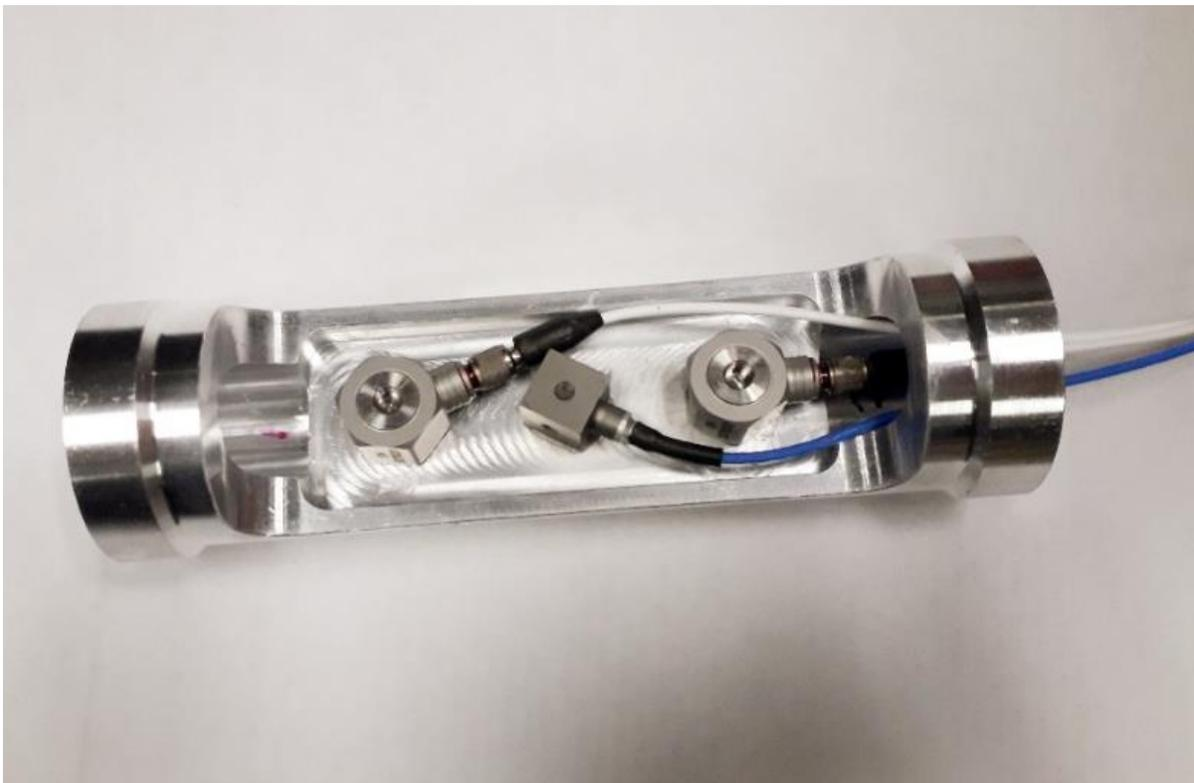
Figure 2.14 The insider view of the instrumented shaker handles showing one accelerometer located in the middle and two uniaxial force transducers located left and right.
