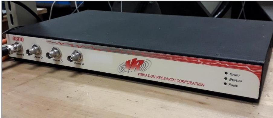
Figure 2.7 The VR8500 vibration control system.
