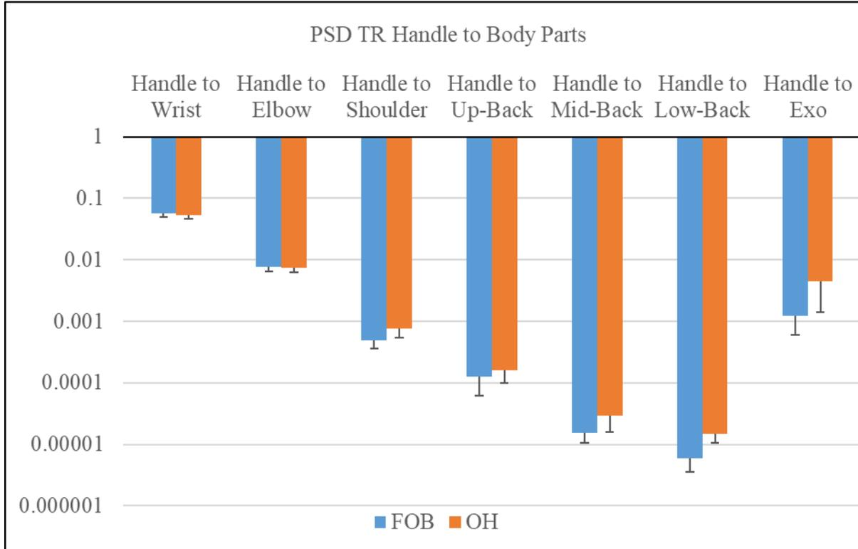
Figure 3.9 Posture effect on PSD transmissibility. OH: overhead posture; FOB: front-of-body posture.
