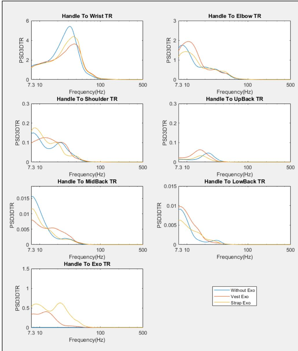
Figure 3.12 Exoskeleton (Exo) effect on PSD transmissibility in the frequency domain.
