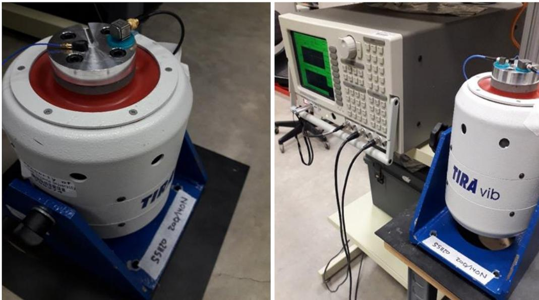
Figure 2.11 Setup for accelerometer base validation
