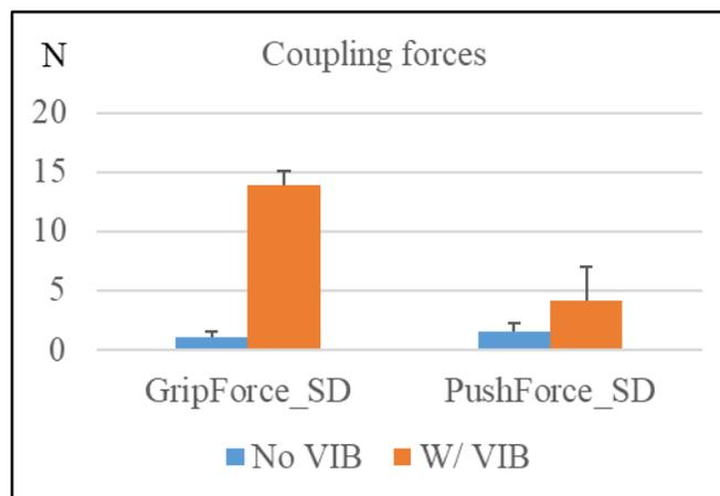
Figure 3.24 Effect of vibration on/off conditions on peak-to-peak coupling forces.
