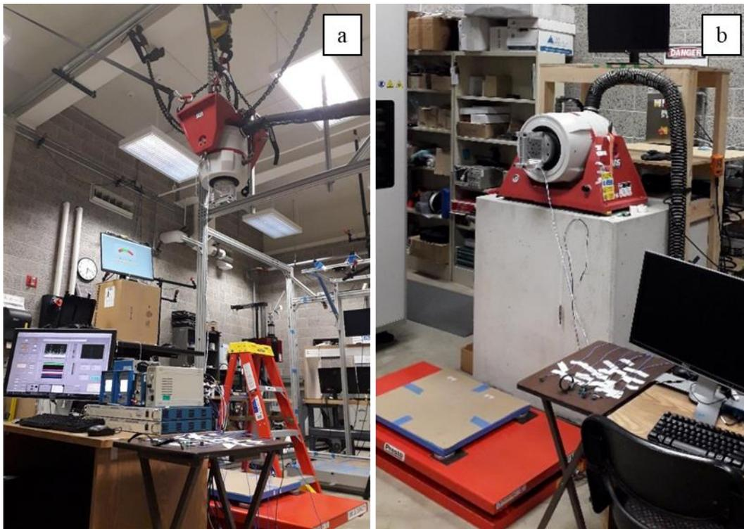
Figure 2.6 Illustration of the electromagnetic shaker setup in the overhead position (a) and the front-of-body position (b), respectively.
