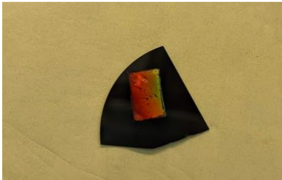
Figure 5.4 HD-DVD grating stamped on silicon substrate using PDMS mold and PMSSQ ink.
