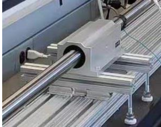
Figure 2- 2: Linear bearing support device [7].
