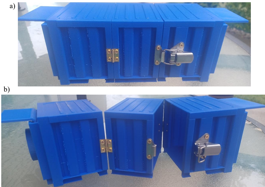
Figure 48: Scaled modified standard container model. a) Side view, b) Opened container view.
