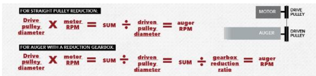
Figure 35: Equations to calculate the rpm of an auger [29].
