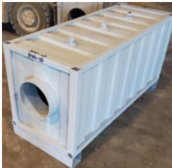
Figure 7: 1/4-scaled shipping container.
