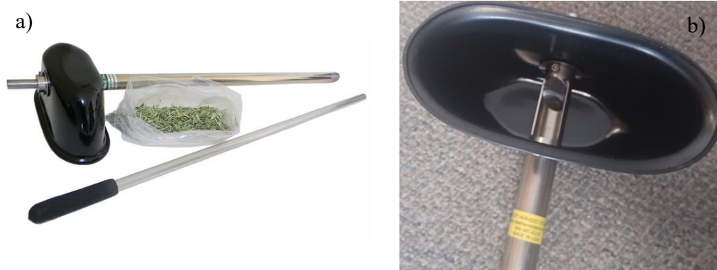
Figure 17: Hay bale sampler probe. a) Components of the bale sampler [22], b) Inside of protective shield with cutout of shaft.
