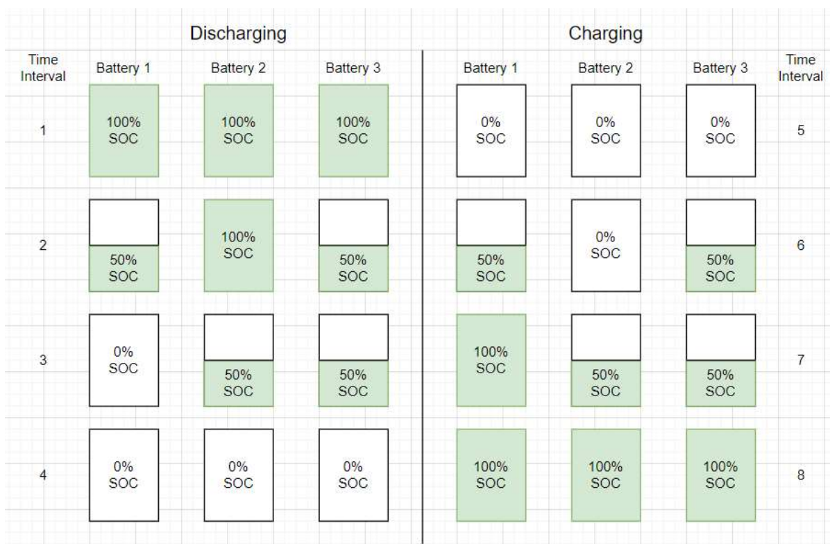
Figure 12: This image shows the charging and discharging pattern of experiment three.
