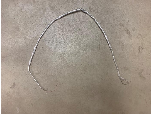
Fig. 3-2: Protected lead wire for strain gauge
