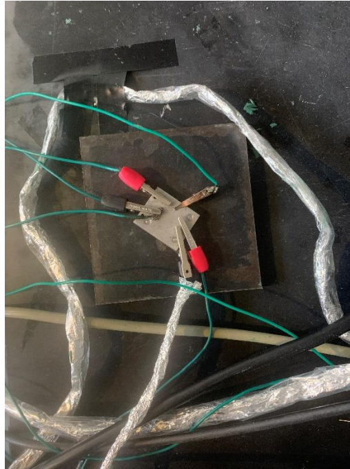
Fig. 3-6: The steel plate used as ground
