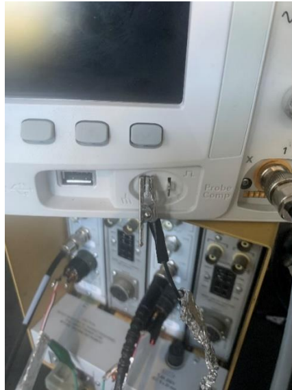
Fig. 3-5: The method for grounding the oscilloscope
