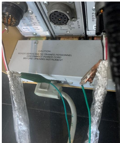
Fig. 3-4: The method to ground the Faraday Cage
