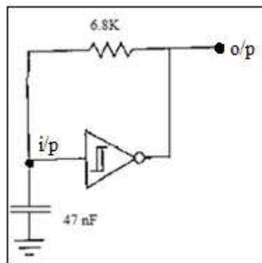
Figure 3.4: Schmitt trigger (in TDR circuit)
