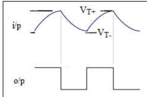
Figure 3.5: Input and Output waveforms of Schmitt trigger ( $V_{T+}$  and  $V_{T-}$  are upper and lower threshold values). [26]
