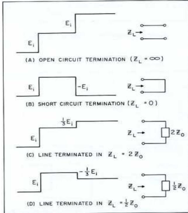
Figure 2.4: TDR displays for different loads. [6]
