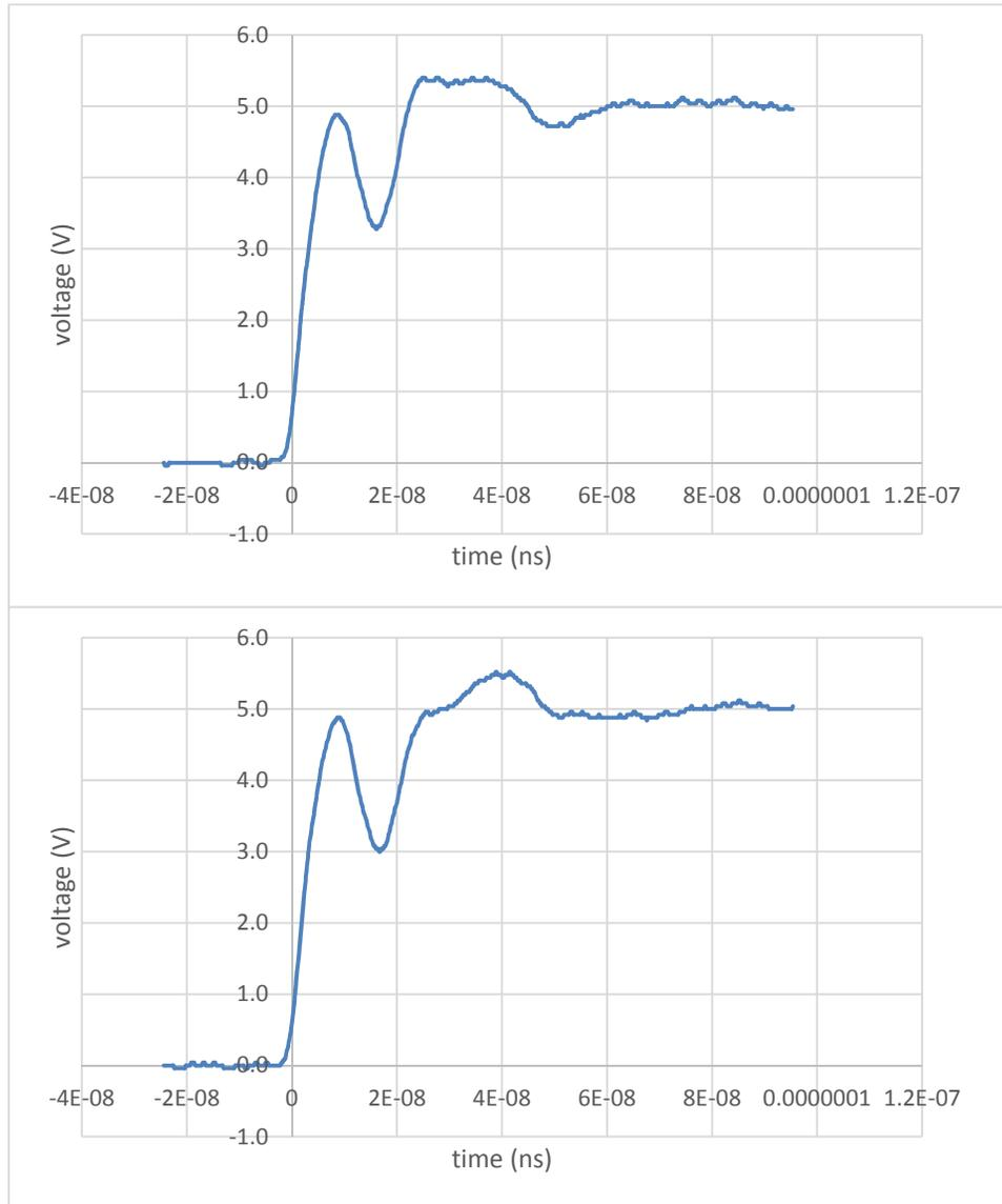
Figure 4.6: a) x-y plot at 400 ml water (13.7 cms), b) x-y plot at 600 ml water (20.3cms).
