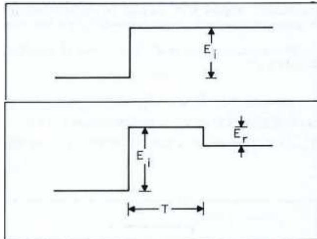
Figure 2.3: (above) Oscilloscope display when load impedance matches characteristic impedance.
