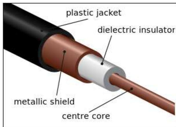
Figure 2.5: Coaxial cable [25]
