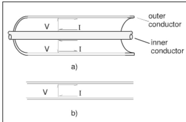
Figure 2.6: voltage pulse propagation through a) coaxial cable and
