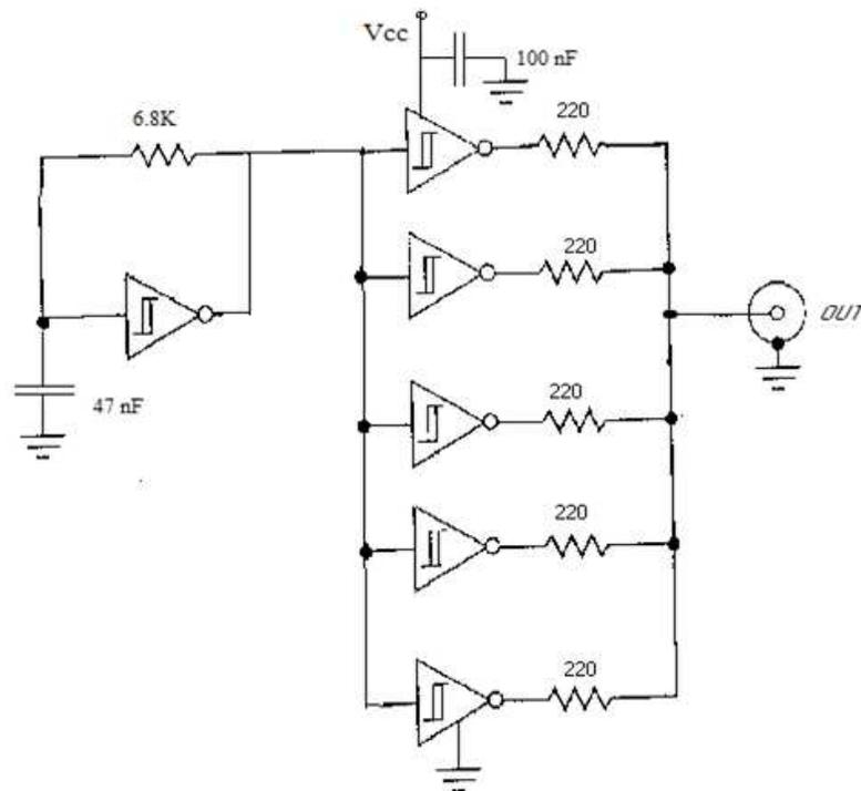
Figure 3.2: Circuit Diagram of TDR circuit [23]
