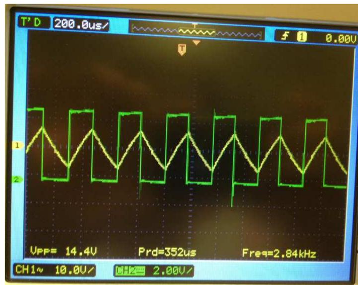
Figure 4.2: Schmitt trigger outputs.
