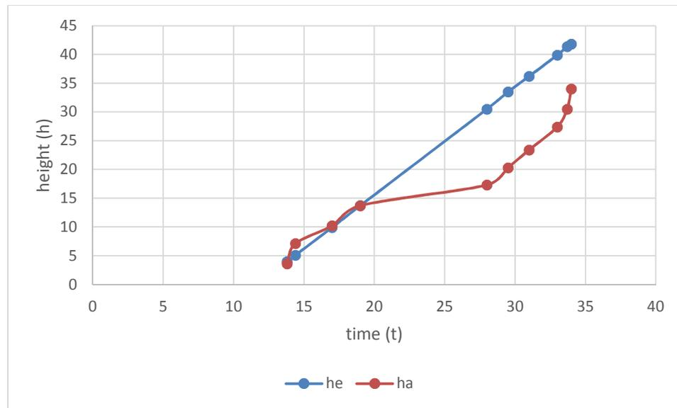
Figure 4.8: a) empirical height vs. time difference, b) actual height vs. time difference.
