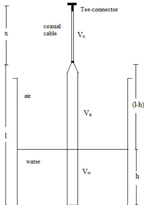
Figure 3.6: Probe setup in the tank.
