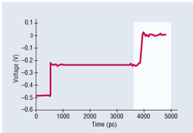
Figure 2.1: A TDR waveform showing the incident signal and the reflected signal (highlighted area). [24]
