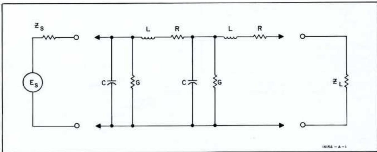
Figure 2.2: Classical model of a transmission line. [6]
