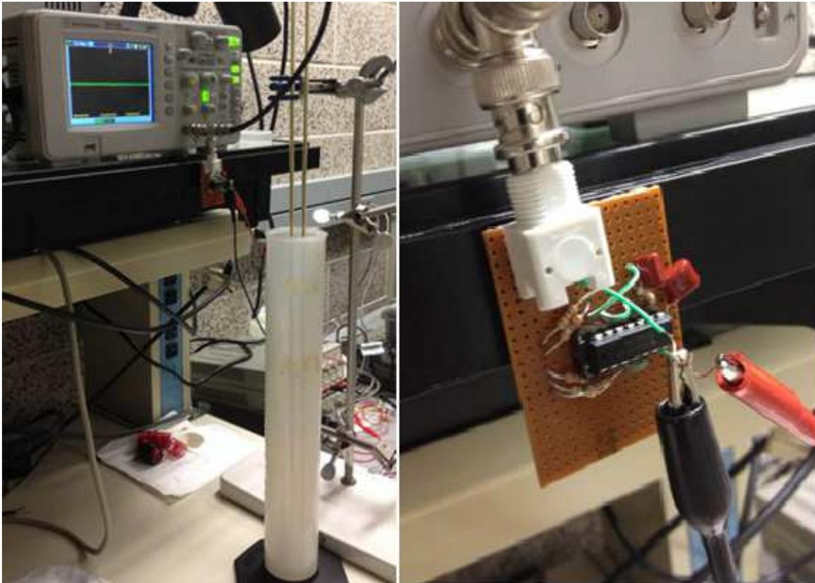
Figure 4.1: a) Experimental Setup, b) TDR circuit built.
