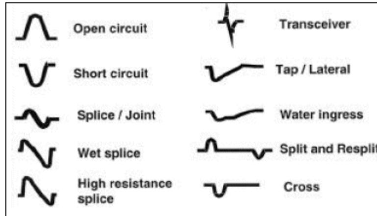
Figure 2.8: Faults and their waveforms. [7]
