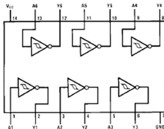
Figure 3.3: Pin Diagram of 74AC14 IC. [7]
