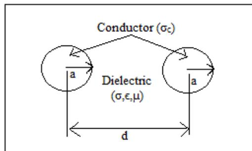
Figure 2.7: Geometry of a 2-wire transmission line [17]
