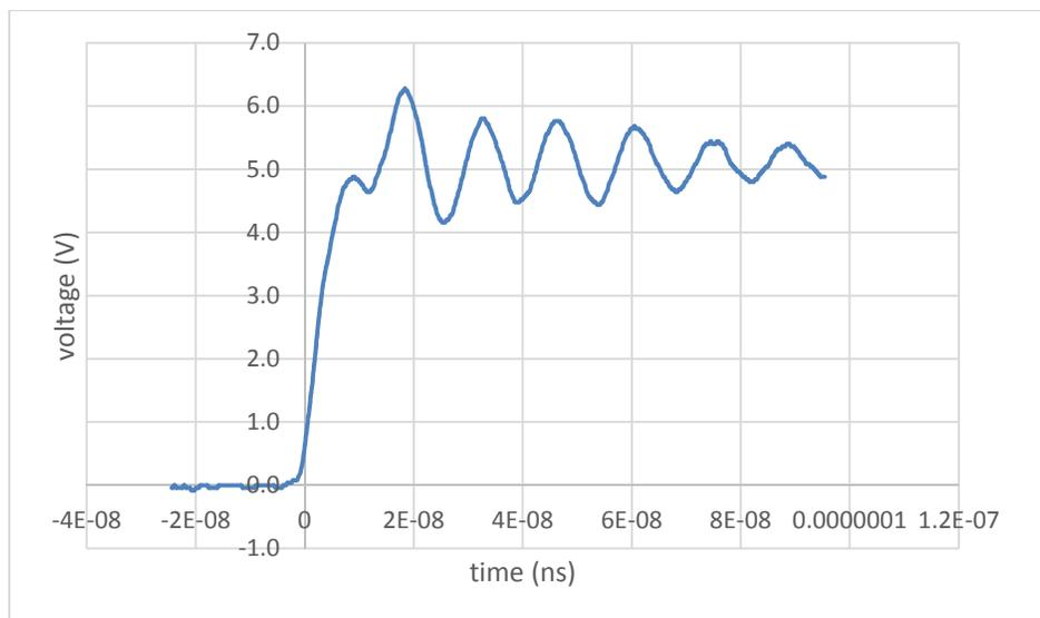
Figure 4.4: Output due to reflection from probe termination.
