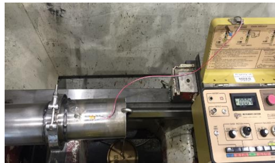
Figure 58 Strain Reading for V band Clamp Support
