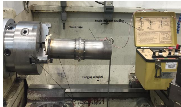
Figure 38 Experimental Setup for Cylinder supported with nut & Bolt
