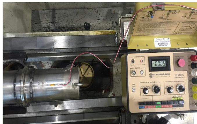
Figure 60 Strain Reading For Nut & Bolt Support
