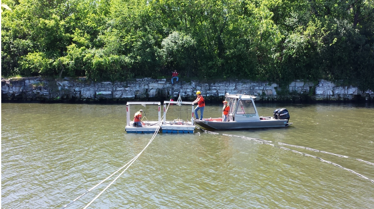
Figure 12. Water guns suspended from pontoon boats in the middle of the canal.
