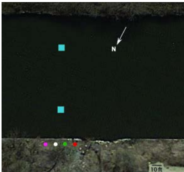
Figure 13. Water gun and geophone configuration for experiment 2
