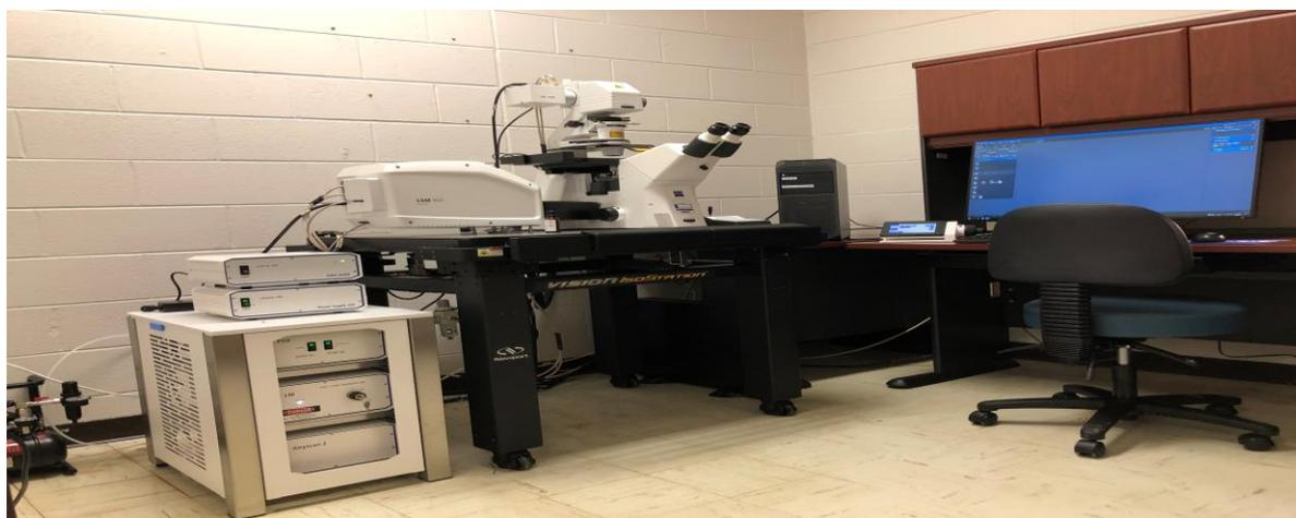
**Figure 1. Zeiss LSM 900 Microscope and set-up.** The confocal laser scanning microscope was used for Airyscan 2 super-resolution imaging. The Zen Blue<sup>5</sup> software was used to acquire z-stacks and generate MIP images of U87 cells and mouse brain sections for automatic segmentation.
