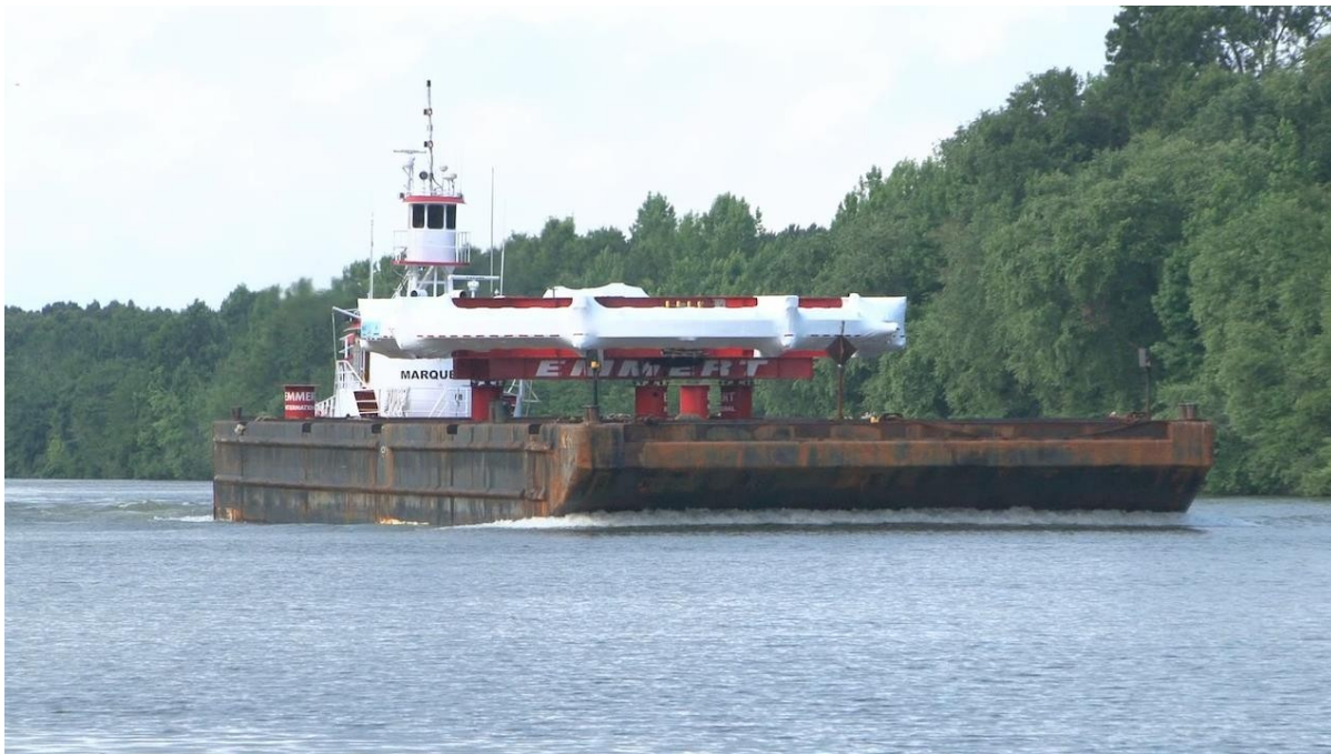
Figure 3.7: The superconducting coils being transported by barge up the Tennessee-Tombigbee Waterway. (Image courtesy of Darin Clifton, Ceres Barge).
