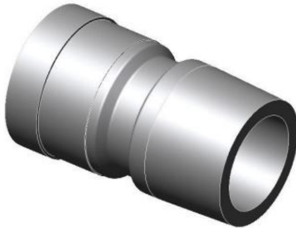
Figure 4.5: A computer drawing of an aluminum end-piece designed to provide an electrical connection between the straw material and the aluminum manifolds holding the straws in place. (Image courtesy of John Carroll, University of Liverpool).
