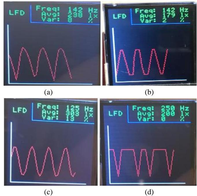
Figure 4. Output plots for (a) fluorescent array, (b) CFL, (c) incandescent, and (d) LED light sources, respectively.
