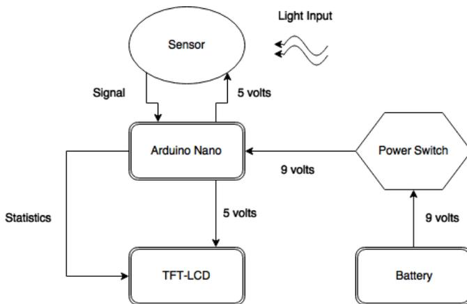
Figure 1. Block diagram of handheld light flicker detector.
