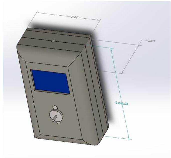
Figure 2. Housing design, exterior.
