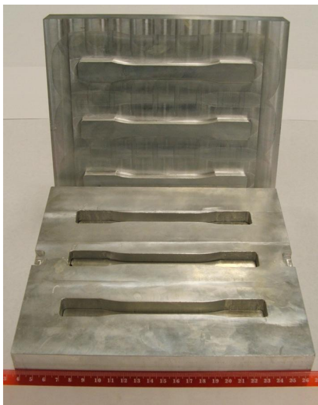
Fig. 2 Three-cavity, aluminum 7075-T651 tensile bar mold in open position; dimensions = cm
