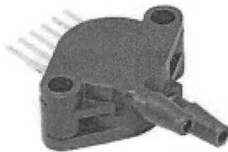
Figure 13: MPX5010DP Differential Pressure Sensor
