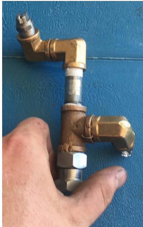
Figure 3.2: Initial Rotary Head Design
