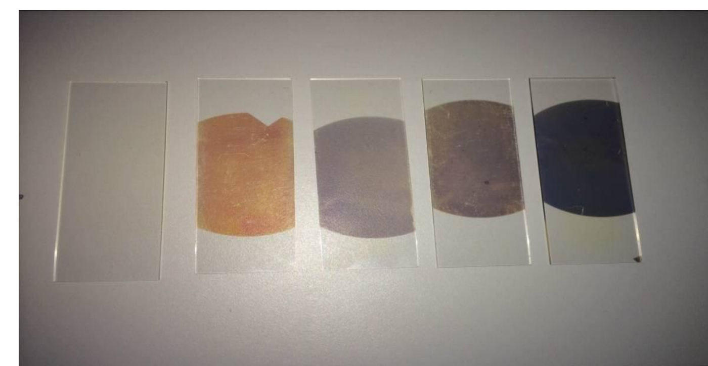
Figure 2: (thin films of Ag deposited and their color intensities observed, with thickness starting from the left with 1.0nm, 3.0nm, 5.0nm, 7.0nm and 10.0nm respectively)
